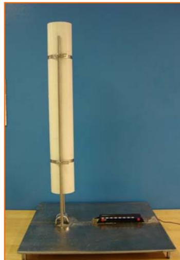
Figure 2- Drop tube apparatus to simulate injury mechanism.
